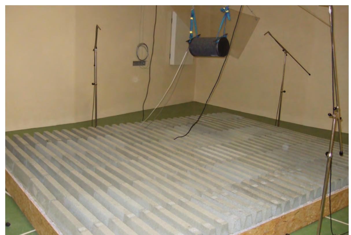
measurement of noise absorption of a protection wall
