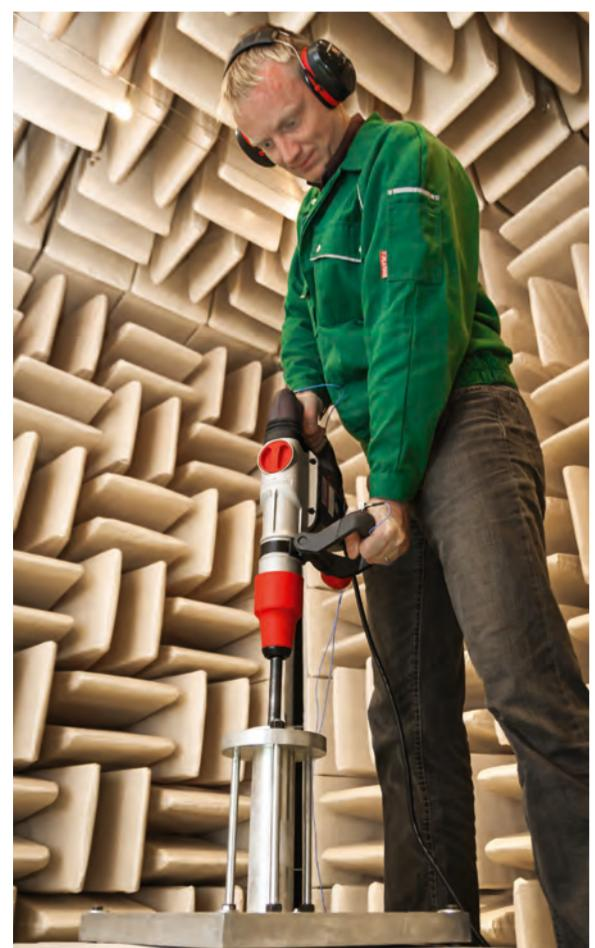
vibration measurement of a percussion drill in loading device
