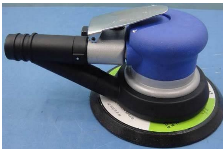
Photo 15: WFS-1039C (tool with dust collect hose and bag)
