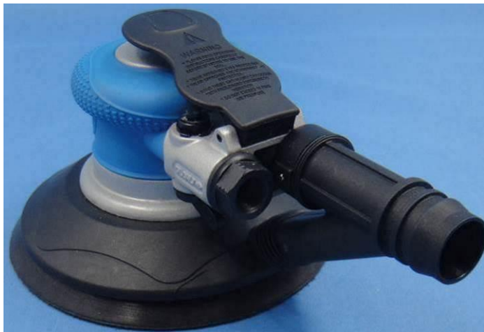
Photo 24: WFS-1338 (tool with dust collect hose and bag)
